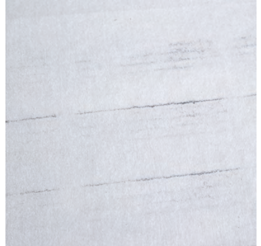
Five decreasing lines of residue followed by clean return stroke
