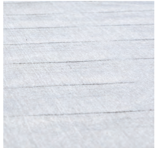
Cleaning effect of successive passes at 40mm per clean
