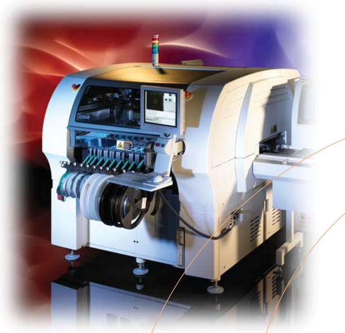
Equipped with two 7-spindle FlexJet3 placement heads and two upward looking cameras for large component image capture, this platform provides high-speed IC placement for high-volume lines or serve the role as a line balancer by off-loading chip placement in lower volume environments.
