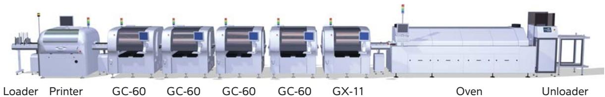
Average Production Capacity: 130,000 - 110,000 cph (0.028 sec/comp) Total Line Length: 16.29 m
