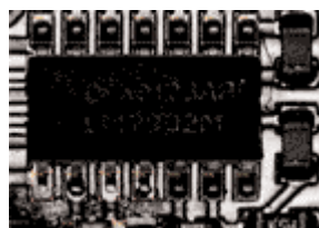
Solder joints DOAL light
