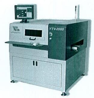
Programming the YTV is fast and intuitive. Operators typically take less than 45 minutes to create a complete inspection program including solder inspection. The YTV utilizes a standard package library to simplify training and insure program portability across manufacturing lines.
