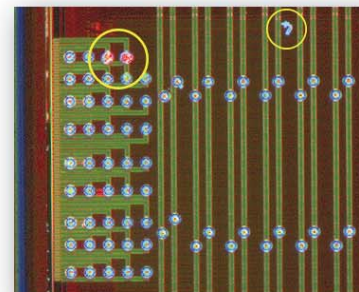
Bump and die defects
