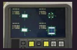
NXT II 's high resolution parts camera can handle parts from 0402 (01005) to large odd-form parts.
