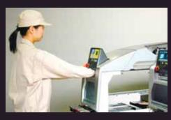
It is possible to quickly perform maintenance operations such as replacing placing heads by pulling out modules. Off-line maintenance is possible by replacing the module with another one, resulting in minimized production
