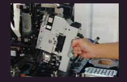
In order to place a wide range of part types, from small chip parts to large odd-form parts, six types of placing heads are available as well as a glue dispensing head. Any one of these easily interchangeable heads can be selected to meet the production needs
