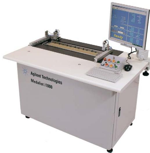
**Press-Down and Vacuum Fixture.** The *Medalist i1000* offers users two different fixture options. The first option uses a typical MDA-type fixture with cable connections. This provides users with affordable fixture options. The second option employs a vacuum-type fixture and a mechanical fixture lock-down system using electrical motors. This cable-less design provides fast fixture swapping time while maintaining high signal integrity.
